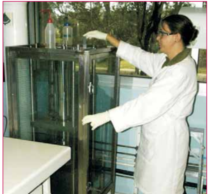
Tanya James, Technical Officer Scientific, prepares to test thrips for insecticide resistance with the aid of a Potter precision spray tower.
