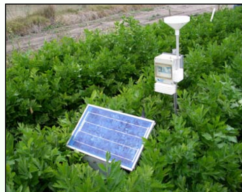
Figure 2. A weather station used in this project. In the foreground is the solar panel unit which also contains the modem and transmitter for sending telemetry via the mobile phone network.
